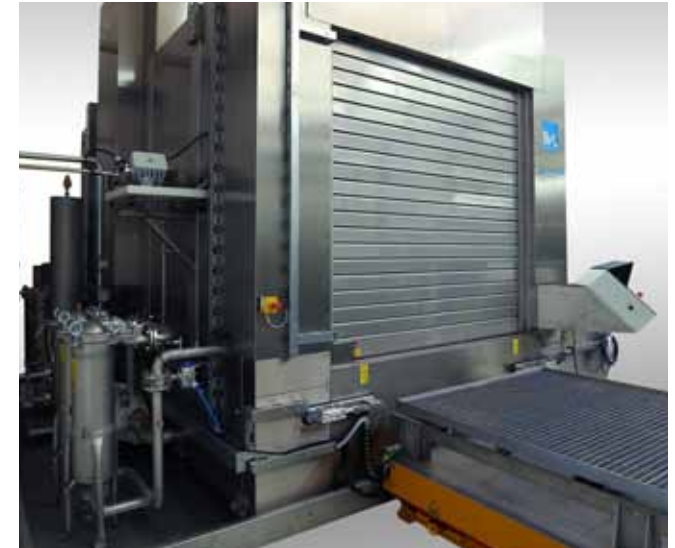
Version PacifictA with rolling gate, filter system and heat exchanger
