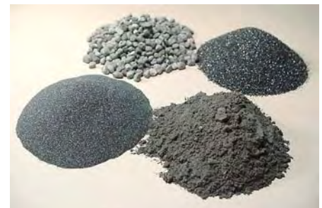
Typical AFM Media abrasives include silicon carbide and diamond abrasives. Particle sizes range from 5 to 4,000 microns (1,000 to 8 mesh).
