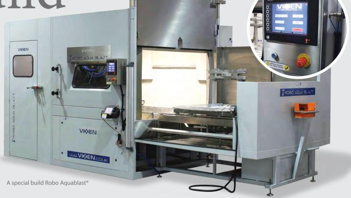
Satellite blasting machine for processing long tubular type components
