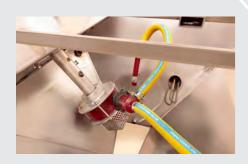
Delivery of the slurry to the hand-held nozzle is via a glandless polyurethane pump and hoses within the machine.
