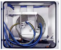
The Aquablast® Tumbler machine featured with 2 stage rinsing, hot and cold, hot rinse not standard. This machine batch processes small parts which are turned in the drum and simultaneously blasted
