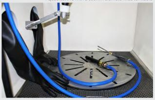
Fixed turntable inside blast chamber
