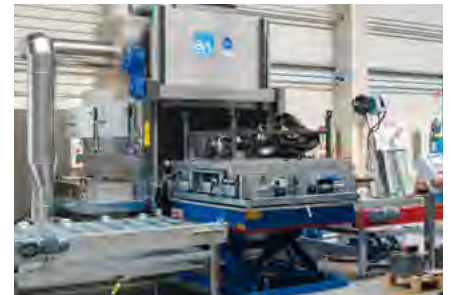
Hydraulic scissor lift table with pneumatic carry in and roller conveyor system
