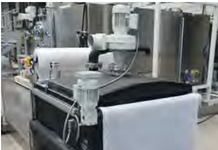
Bath maintenance: Belt filter
