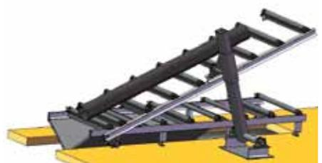
*Tilting device for pipes to evacuate the abrasive after blasting*
