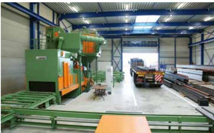
*Crossover conveyors connect the roller conveyor blast machine with the sawing and drilling machines.*
