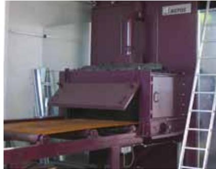
*Blast machine for metal sheets*
