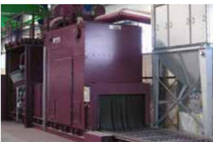
*Blast machine for metal sheets, sections and constructions with a passage height of up to 1000 mm*
