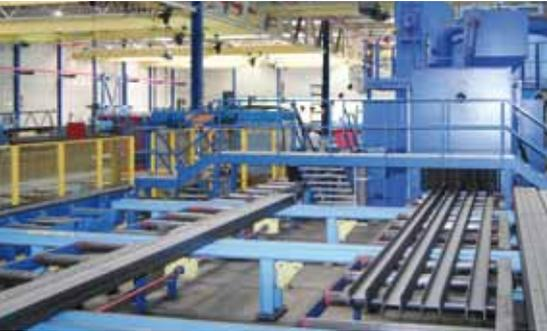
*Blast machine with crossover conveyors*
