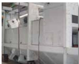
Machine housing with blast chamber made of manganese steel
