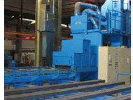
*Blast machine with adjustable passage height*
