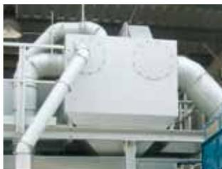
Baffle case for the separation of coarse particles
