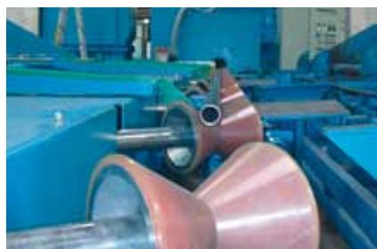
*Diabolo blast machine for handling sprinkler pipes*
