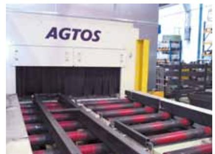
*Blasting machine with adjustable passage height*
