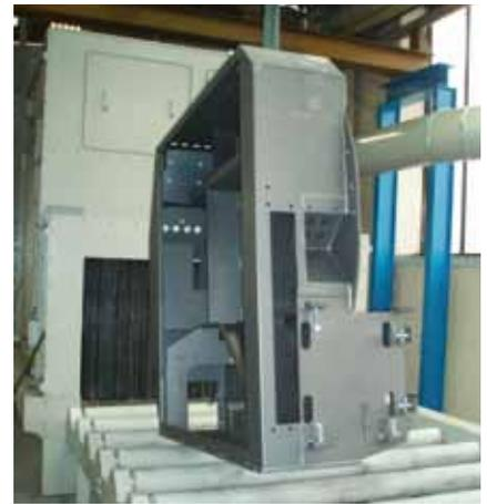
*Blast machine for metal sheets, sections and constructions with a passage height of up to 1000 mm*
