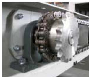
Pedestal bearings of the rollers are installed outside the machine
