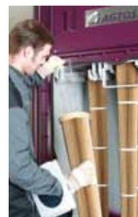
Quick and easy exchange of filter cartridges
