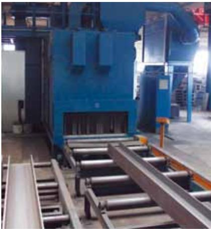
*Blast machine for large sections*
