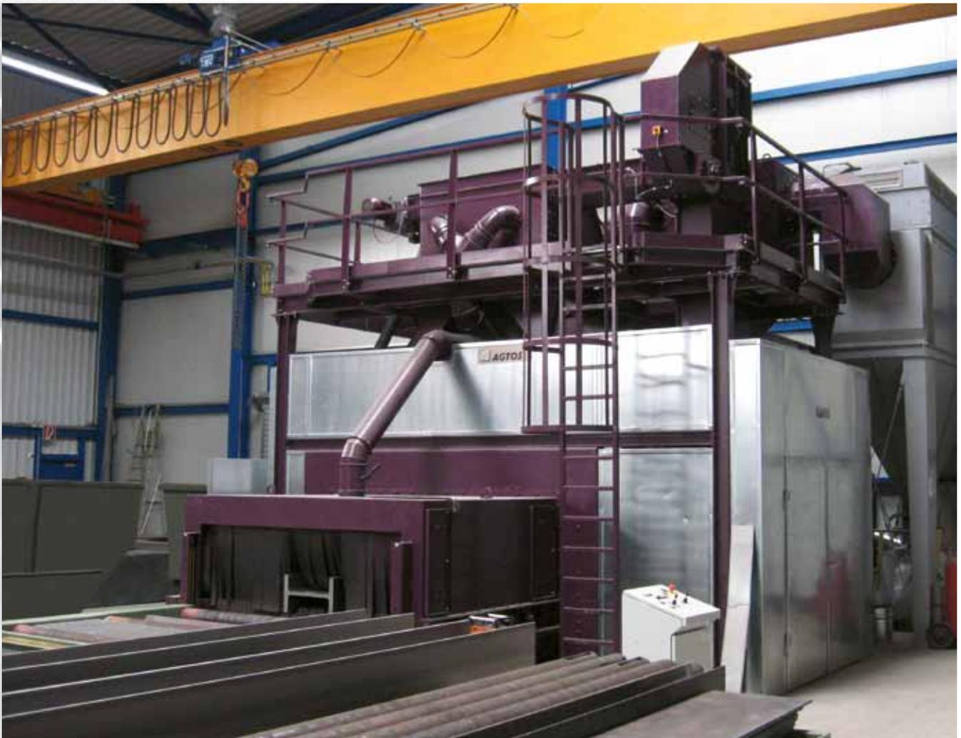
Roller conveyor blast machines are used to remove scale and rust from metal sections, metal sheets and constructions. By combining a roller conveyor with the appropriate cross-over conveyors, individual process steps such as blasting, conservation, sawing and drilling can be interlinked. This ensures a flexible manufacturing process and a high material rate.
