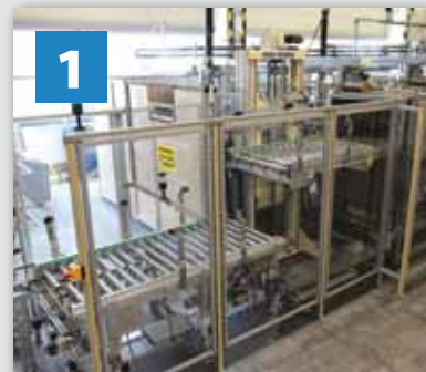
Detail Hub-Senk-Station
